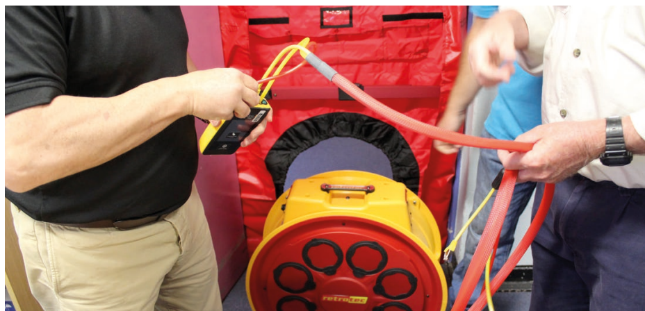
The blower door test rig allows for testing of a building's air leakage rate.
